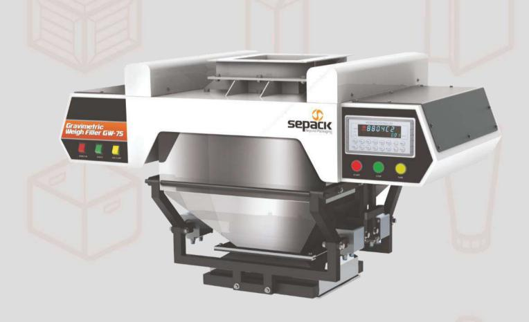
Gravity feed, Vibrator feed, and Screw feed systems are available to suit specific product requirement.
